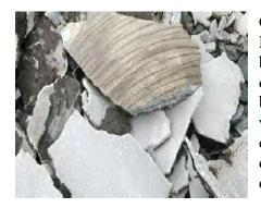
Figure 2. Struvite Buildup Removed From Pipe
