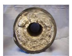
Figure 1. Struvite Blockage in Digester Overflow Piping
